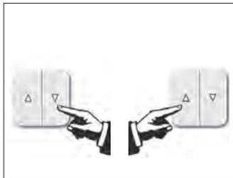
Extend the awning with the ▼ (DOWN button) until the front rail stop can be operated.
